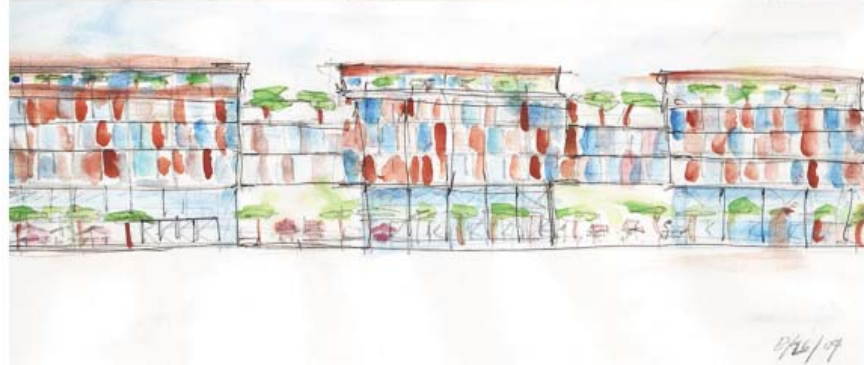
Initial Conceptual Sketches Developed Park Program and Elevation Demonstrating Communal "Outdoor Bridges/Terraces" and Customizable Sliding Panel / "Second Skin" System
